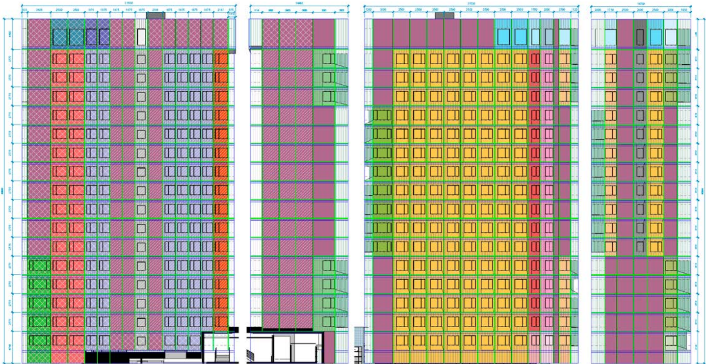
Façade setting out for Building B
