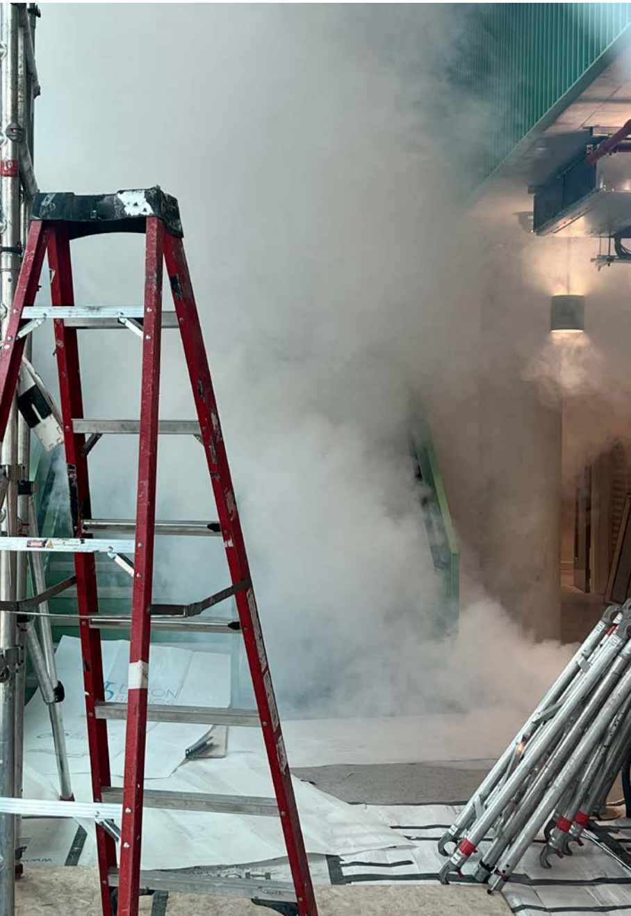
Smoke machines in action Observation of leakage through louvers at podium level
