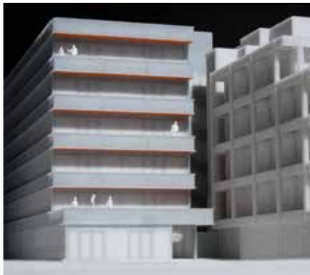
Depth of facade creates solar shading and occupant amenity
