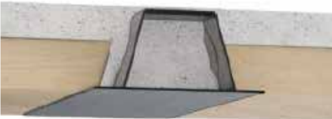
2 Delta beam system set into concrete planks
